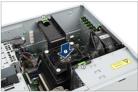
Figure 37: Installing system fan 2 (and 4)
